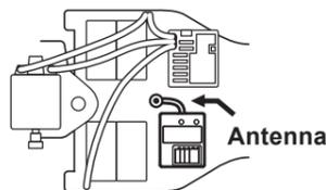
**Installing the Antenna**
